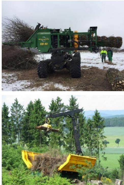
behind the forwarder. Most of the time is lost on loading, so it is of great importance that the harvester places the cut trees in an optimal position for collection.
